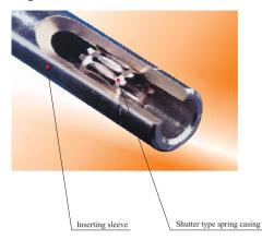
Explosion-proof plugs and sockets have the feature of self-cleaning. An elastic shutter type spring casing is mounted in the inserting sleeve of the socket, which ensure low contact resistance and low temperature rise while reducing the force of inserting and pulling.
