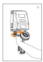
▲ Turn right the plugs, when hearing the sound of "kaca", while the power is connected. In this case, it's impossible to pull out the plug from the socket. Last revolve the plug and lock it on the socket to comply with the requirement of IP66.
